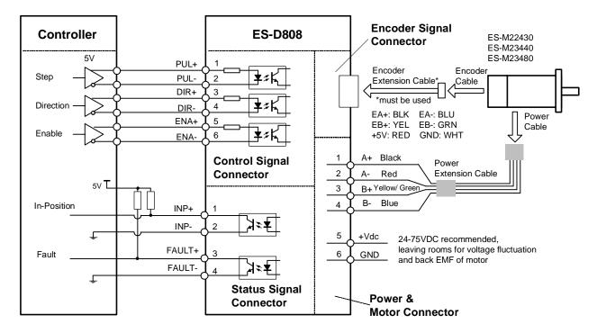
Connections to controller of differential output
