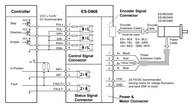
Connections to controller of sourcing output
